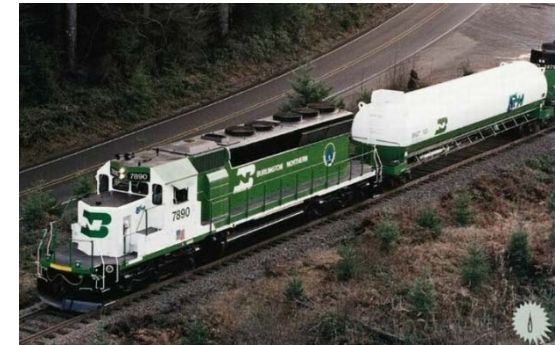
Dual diesel/LNG powered train - USA
