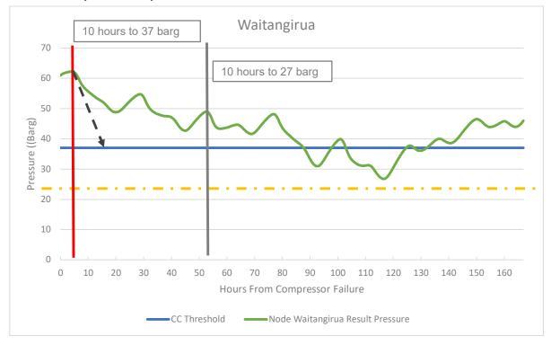
Similar examples exist throughout the transmission system. With the current CC pressure ranges, there is a risk of unnecessary or premature curtailment.
