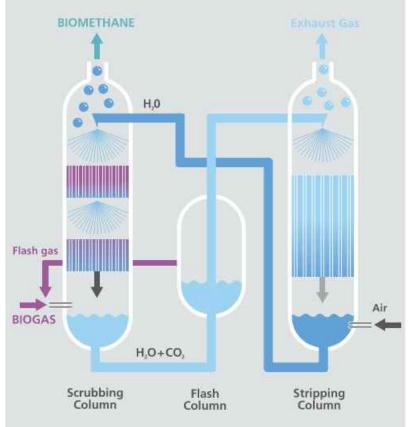
Figure 13-7: Scrubbing technologies schematic (UNIDO & German Biogas Association, 2017)
