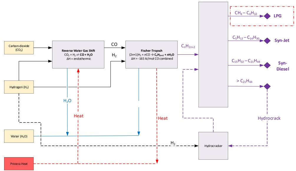
Figure 13-9: Process Schematic of Fisher-Tropsch Process
