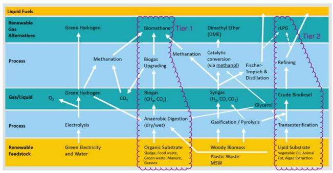
Figure 2-1: Summary of Production Pathways, Including Feedstocks, Processing Technologies, and Products \*Plastic waste and MSW are not renewable feedstocks but can be utilised in Waste-to-Energy applications The pathway from biogas to syngas (i.e., biogas reforming) has not been considered, as the key driver is to transition the natural gas network, and biogas represents a more valuable intermediate than syngas.
