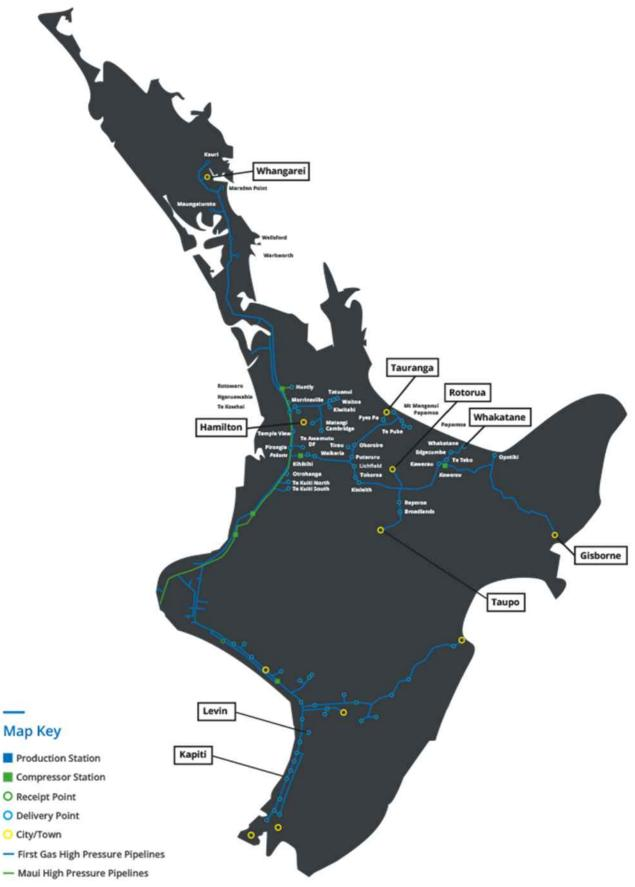
Figure 3-1: Existing Natural Gas Reticulation Network (First Gas, n.d.)
