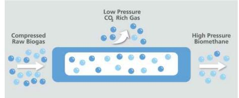
Figure 13-8: Membrane Separation Fundamental (Pentair Haffmans)
