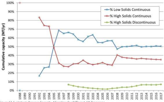
Figure 13-5: Historic Process Capacity Allocation for Different AD Processes
