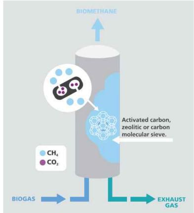
Figure 13-6: PSA sieve pressurization (UNIDO & German Biogas Association, 2017)
