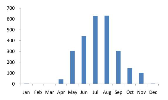
Figure 67: Concept modelled monthly kWh heat load distribution for a medium Wellington heating load
