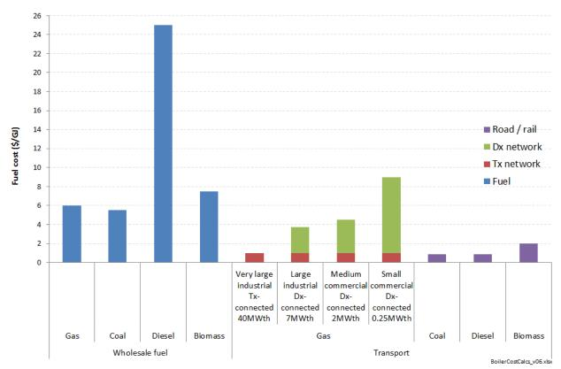
Figure 40: Fuel and transport costs for different boiler options
