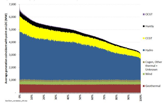
Figure 64: Average generation coincident with point on load duration curve for 2011
