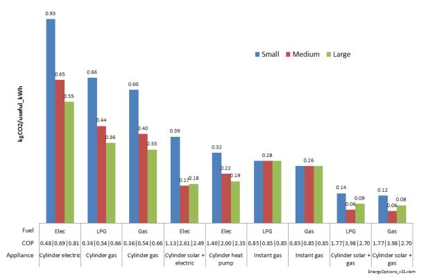
Figure 11: CO<sub>2</sub> emissions intensity of water heating options (kgCO<sub>2</sub>/useful\_kWh), assuming a central electricity emissions intensity scenario for small, medium, and large domestic water heating loads
