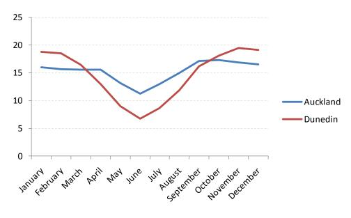
Figure 4: Average daily MJ solar water heating for a typical solar panel in two representative locations
