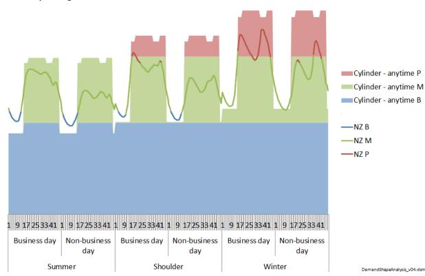
Figure 77: Illustration of the classification of cylinder-based heating demand into baseload, midmerit, or peaking
