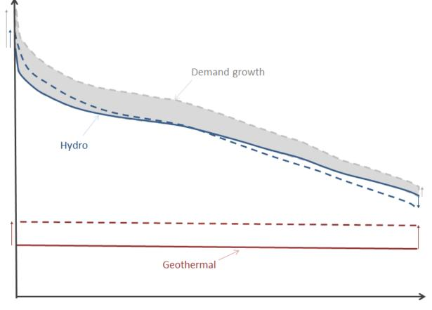
Figure 66: Illustration of hypothetical combination of geothermal build plus increased sculpting of hydro to meet peaky demand growth
