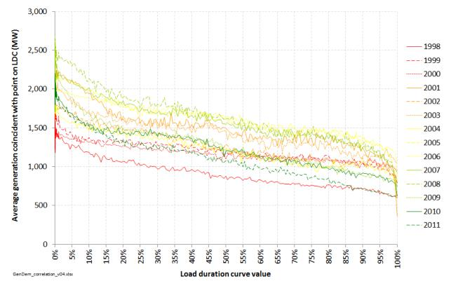
Figure 72: Average thermal generation coincident with point on the national load duration curve
