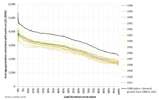
Figure 71: Average hydro generation coincident with point on the national load duration curve
