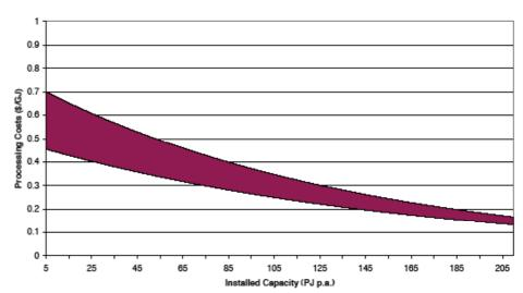
Gas Processing Costs vs Installed Capacity (10% discount rate)
