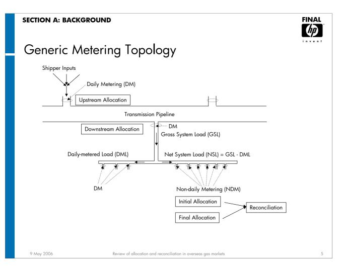
Physically, all gas markets are broadly similar. Producers "input" gas into a high pressure transmission pipeline or pipeline network. Gas is then taken off at "offtake points" and delivered into a distribution network. From this network, gas is delivered to individual customers.
