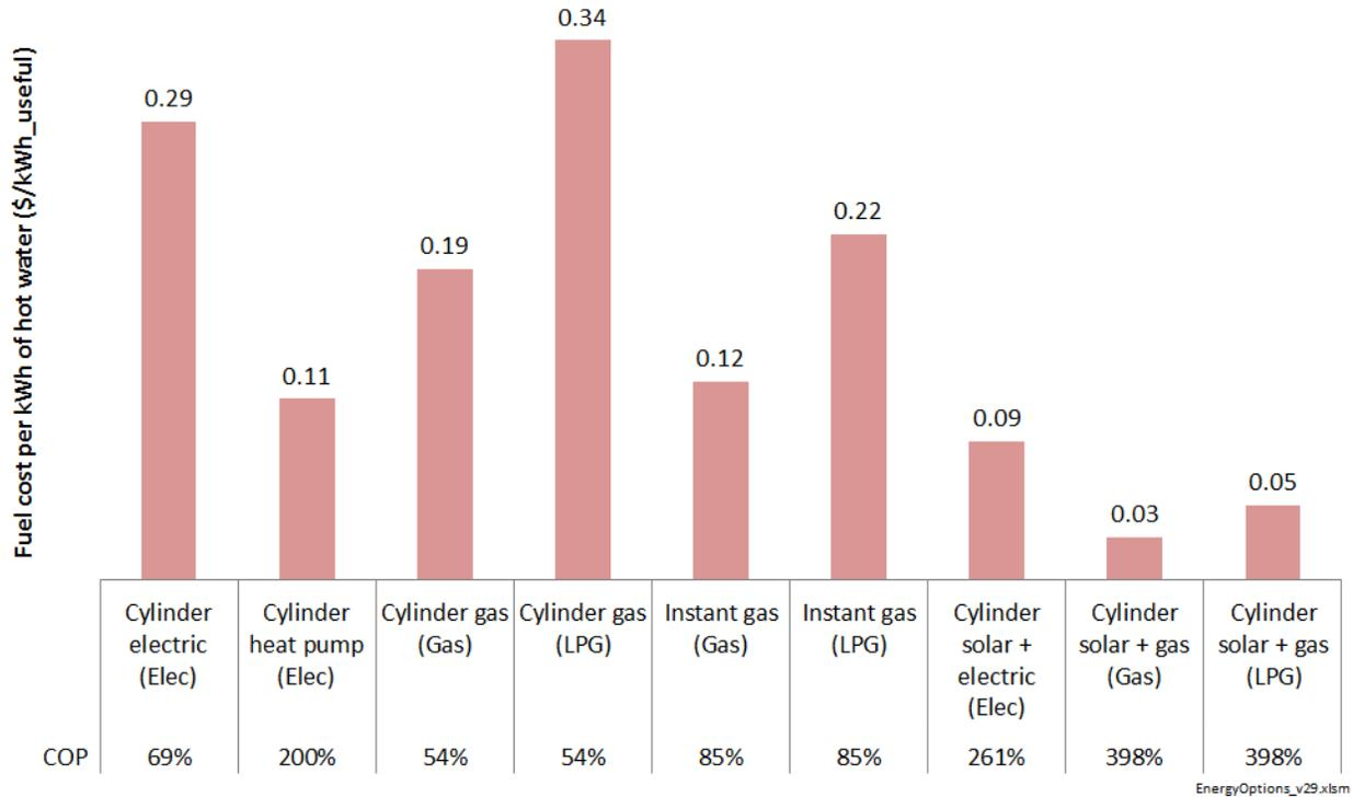
As can be seen, purely on a \$/kWh variable fuel cost basis (i.e. ignoring capital and maintenance costs), solar and heat pump water heaters are the cheapest options, even though electricity is one of the most expensive fuels.
