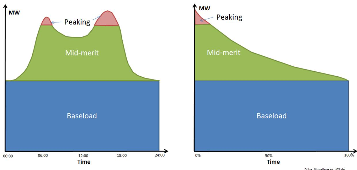
In Figure 62, the diagram on the left shows a chronological representation of how demand varies over time (in this case a single day), and the diagram on the right shows how this demand can be reordered in a load duration curve format.
