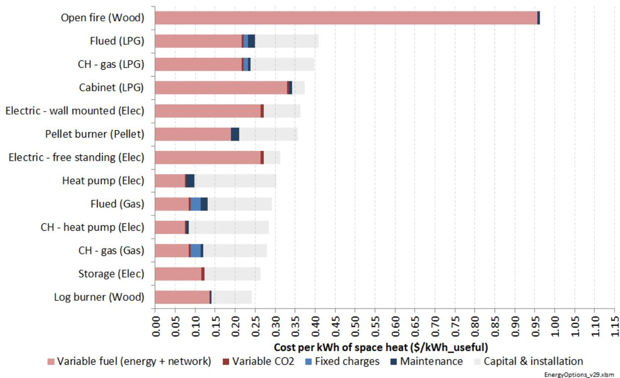
As can be seen, although the variable fuel & CO<sub>2</sub> costs are identical to the small heat load situation represented in Figure 32, the effective contribution of capital and fixed costs is much lower. This makes lower running cost but high capital cost options such as log burners, gas-fired heaters and heat pumps more cost-effective.
