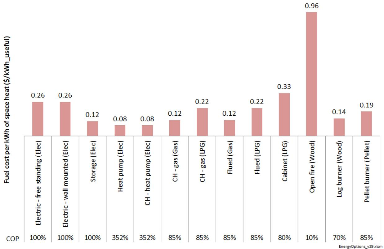
As can be seen, purely on a \$/kWh variable fuel cost basis (i.e. ignoring capital and maintenance costs), heat pumps are the cheapest options, even though electricity is one of the most expensive fuels. Open fires are so expensive to heat a property because they are only 10% efficient.
