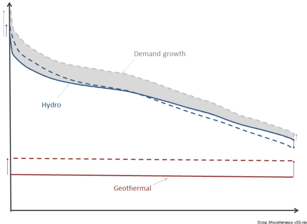
In Figure 66 the solid blue and red lines represent the hydro and geothermal generation profiles at the start of the period, and the dashed lines represent their respective generation profiles at the end of the period (e.g. after ten years) in order to meet the peaky demand growth represented by the grey shaded area.
