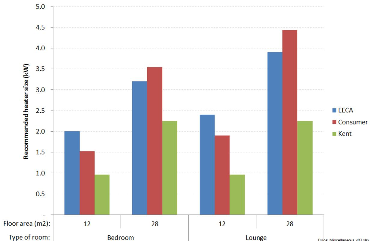
As can be seen, there is not only variance in the size of heater recommended for different room situations, but the rate of increase in the required heater size with room size varies between organisation. Thus, Consumer and Kent have the required heater size increasing in direct proportion to the room size, whereas EECA has the required heater size increasing at 70% of this rate. It is not known what is driving these significant differences between these different organisations.
