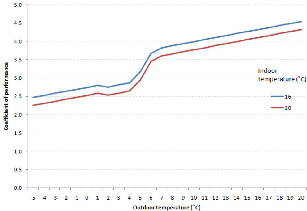
It should be noted that some of the most modern heat pumps have COP curves which are superior to the one shown above, in particular with minimal COP drop-off around the dew point, but equally some also have COPs which are inferior.
