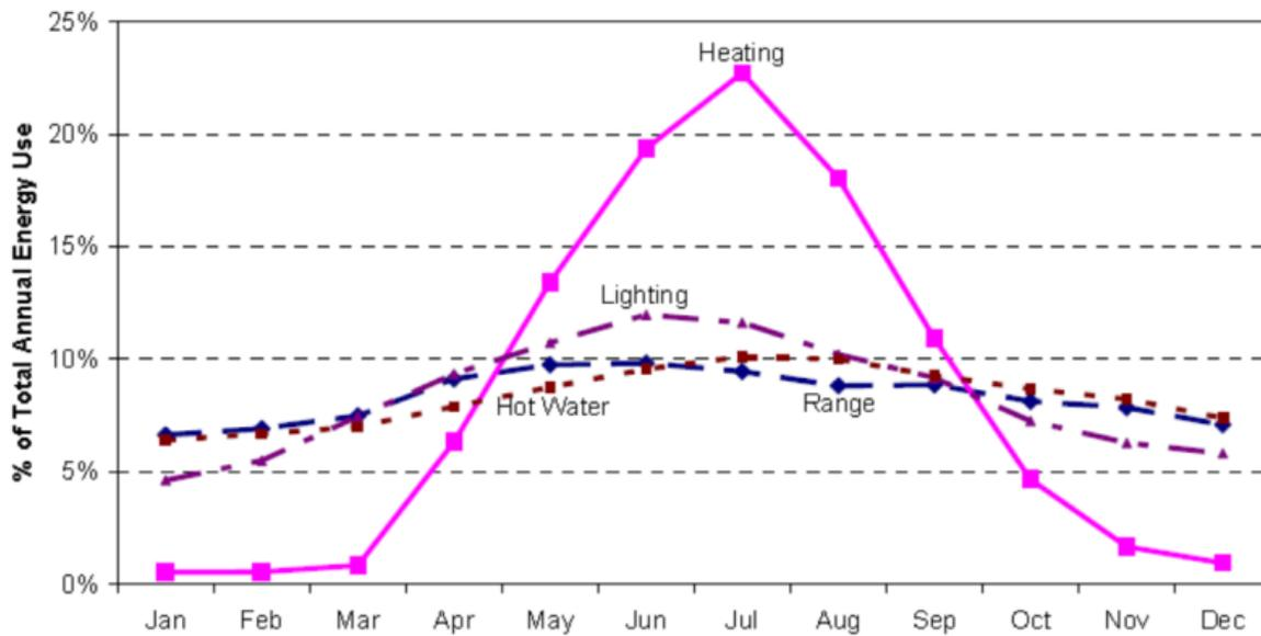
This monthly profile was cross-multiplied with a within-day water heating profile based on research published by Meridian and shown in Figure 3 below:
