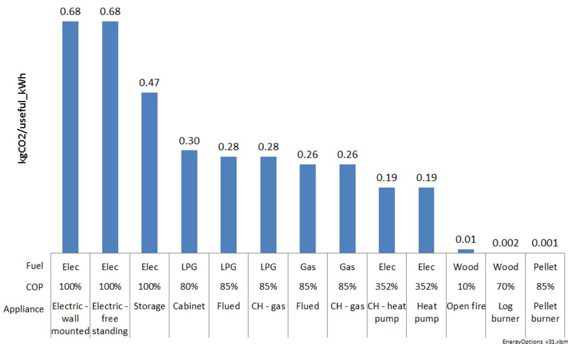
Source: Concept analysis. Note: The heat pump COP chosen is for a Wellington location.
