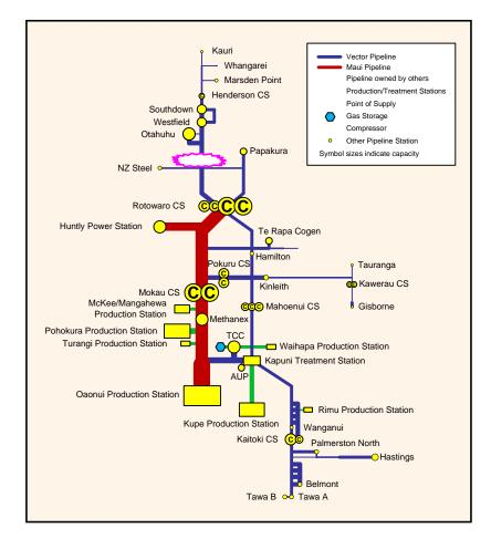
As can be seen from the schematic, there are no pipelines that bypass the damaged and isolated section. As a result, and due to the small amount of linepack in the north system, very rapid curtailment would be required so as to ensure that the distribution networks in Auckland and points north did not become depressurised.
