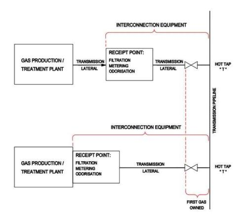
The most common *Delivery Point* configuration is shown in Figure 3. Either party may own the *Delivery Point*, but First Gas will always own the physical connection to its transmission system.
