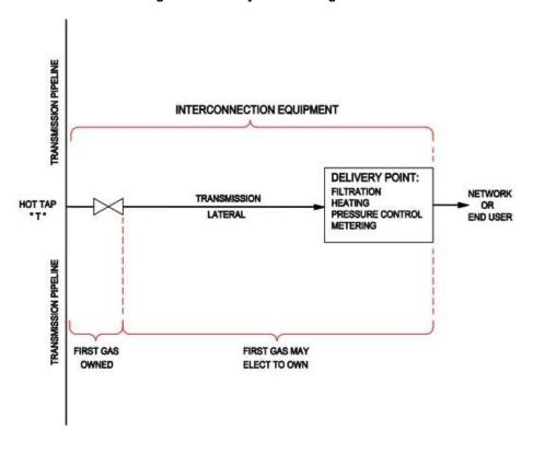
**Figure 3: Delivery Point Configuration**
