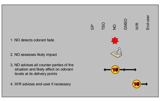
Figure 5 – communication when odorant fade is detected
