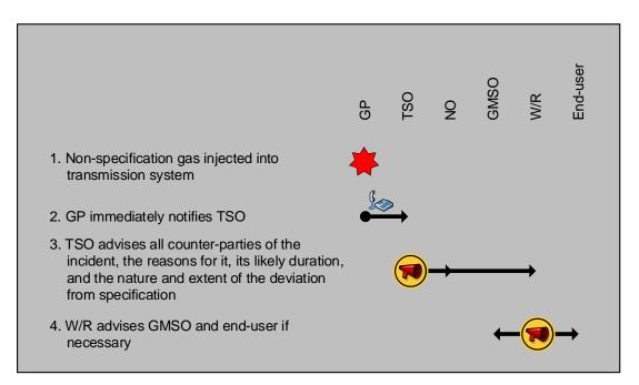
Figure 3 – communication during a gas specification incident
