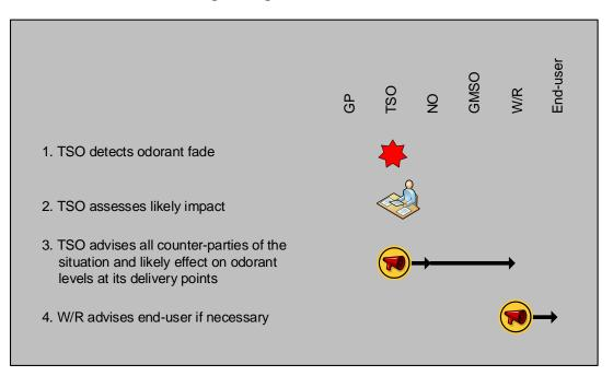
Figure 4 – communication when an odorant plant fails
